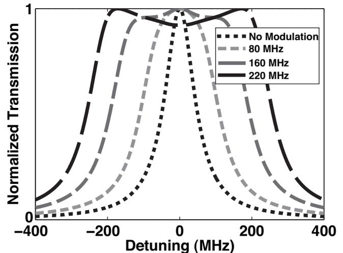
FIG. 2. The effect of laser modulation on atomic transmission resonance. The modulated laser spectrum [Eq. (1)] is convolved with an exponentiated Lorentzian line shape. As the modulation amplitude increases, the top of the resonance flattens and then sidebands begin to appear.
