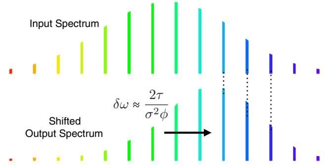
FIG. 2. Graphical depiction of input and output spectrum of the anomalous weak values interferometer. The comb teeth have not shifted, but the amplitudes have changed. It should be noted that the output spectrum will be considerably weaker than the input spectrum.
