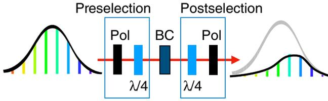
FIG. 1. Experimental schematic. An optical frequency comb spectrum is placed in an anomalous weak value configuration. A preselected state is chosen using a combination of a polarizer (Pol) and quarter wave plate ( $\lambda/4$ ). A birefringent crystal (BC) imparts a relative phase time delay for each polarization. For simplicity, it is assumed that no transverse walk-off occurs in the crystal. The postselection is made with a second quarter wave plate and polarizer.
