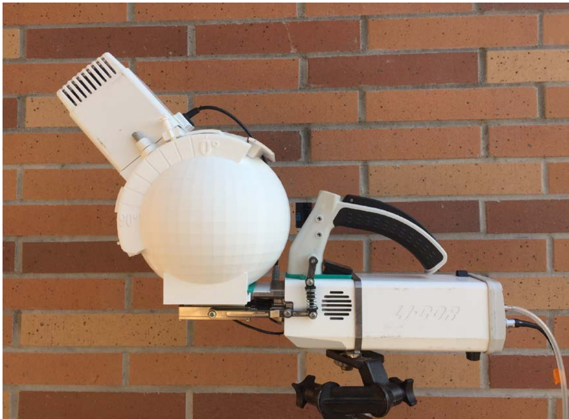
Figure 2. Image of the LI-6800 large leaf chamber and light source attached to the integrating sphere. As seen, the light source is mounted at approximately 45° along the track. Photo credit: Gregory R. Goldsmith.
