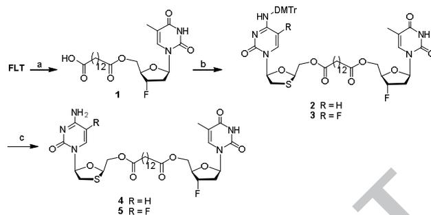
**Scheme 1.** Synthesis of unsymmetrical 5',5'-dinucleoside 1,14-tetradecanoate esters of FLT with FTC (**4**) and 3TC (**5**): (a) 1,14-tetradecandioic acid, HBTU, DIPEA, DMF, rt, 4 h; (b) 3TC-DMTr/FTC-DMTr, HBTU, DIPEA, DMF, rt, 6 h; (c) TFA in acetic acid (2%, v/v), rt, 1 h.
