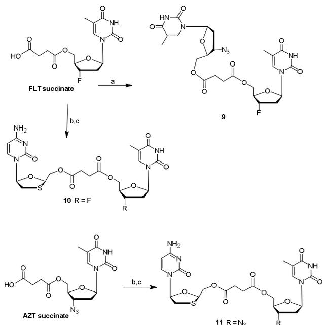
**Scheme 3.** Synthesis of unsymmetrical 5',5'-dinucleoside 1,4-succinate derivatives of FLT, AZT, and 3TC. (a) AZT, HBTU, DIPEA, DMF, rt, overnight; (b) 3TC-DMTr, HBTU, DIPEA, DMF, rt, overnight; (c) acetic acid (80% in water, v/v), 80 °C, 1 h.
