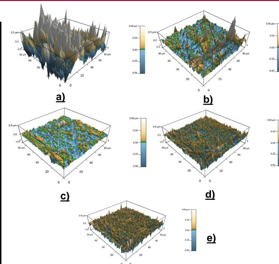
**Figure 5.** AFM images of the gold sample after each step of preparation
