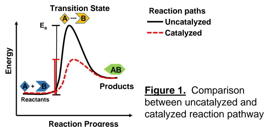
Metallic catalysts are especially important in reactions involving gaseous molecules. Due to their rapid movement and overall low density, it is difficult for gaseous molecules to effectively collide and react. Metallic catalysts provide a surface interface where molecules can arrange and form bonds more efficiently.
