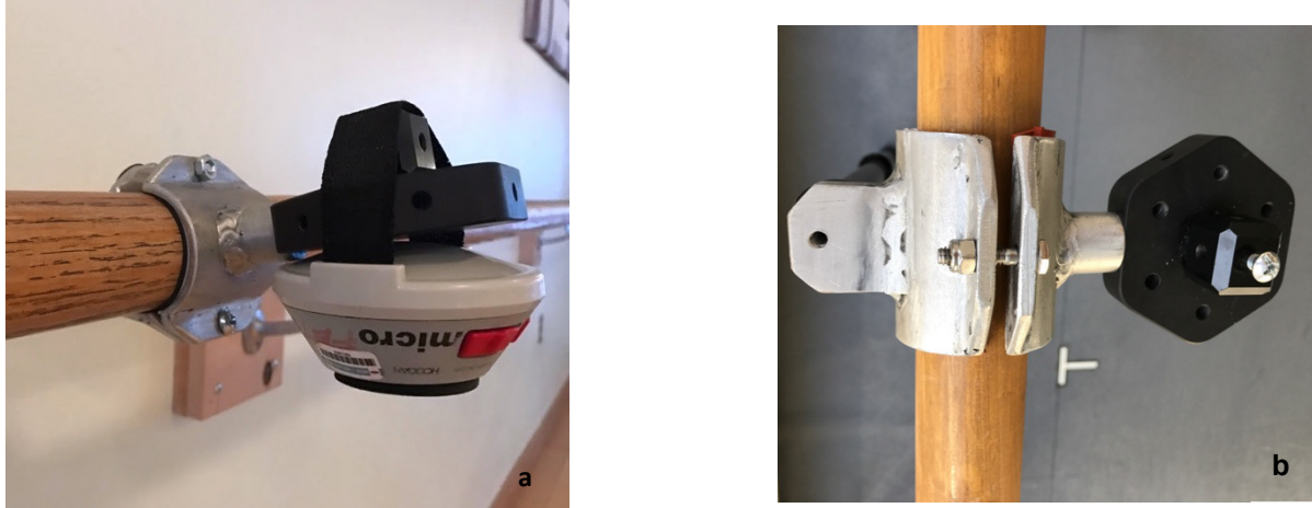
405 FIGURE 1a-b: DynaRail anchoring system and Hoggan Scientific, LLC. microFET®2 digital handheld 406 dynamometer muscle tester. The dynamometer is attached to the disc device with Velcro squares and 407 elastic band. 408
