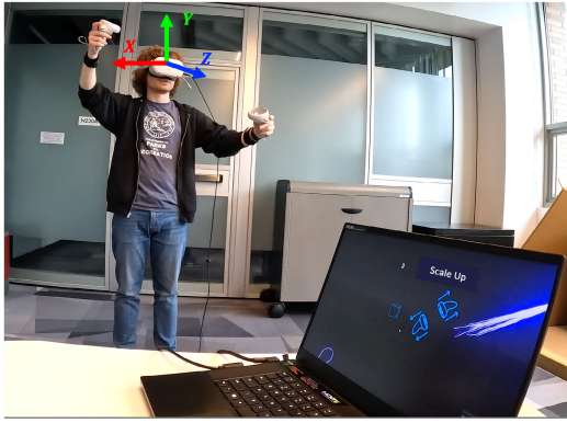
FIGURE 2. A participant was performing a dual-hand interaction gesture - Scale-Up using Meta Quest 2; the VR system for data collection showed the participant each interaction gesture using an animated visual prompt.
