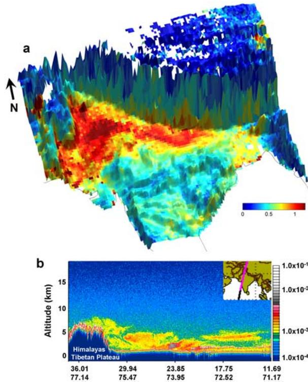
**Figure 2.** (a) Mean MODIS AOD, during pre-monsoon period 2003 to 2006, projected as a function of surface topography, and (b) CALIPSO backscatter profile from Southern India to the Himalayas, reveals the vertical extent of aerosols at elevated altitudes (>5 km) piling up against the slopes of the Himalayas. Inset image shows the lidar transect on 12 May 2007. Backscatter signal from aerosols usually lie in the Yellow-Red color scale and clouds are marked by pink, grey and white colors.
