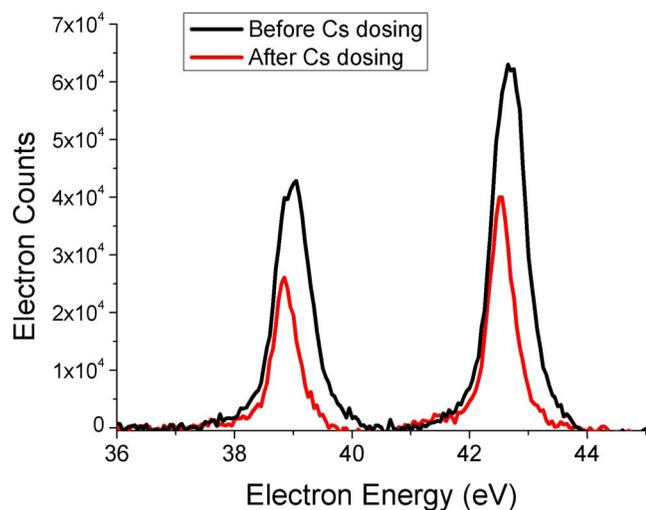
FIG. 4. (Color online) Attenuation of the Au 4*f* XPS peaks. The red peaks are the photoelectron energy distribution of the Au 4*f* XPS peaks before dosing and the black peaks are after Cs dosing. The background has been subtracted from the data for better comparison.
