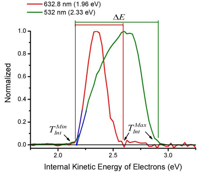
FIG. 2. (Color online) Photoelectron energy distribution of a cesiated Au(111) sample from 632.8 and 532 nm lasers. The work function of the surface ( $\Phi_{Cs/Au}$ ) is found by subtracting  $\Delta E$  from the energy of the photon. The value of the internal kinetic energy of electrons where the blue lines intersect the x axis determines the value of  $T_{int}^{min}$ .
