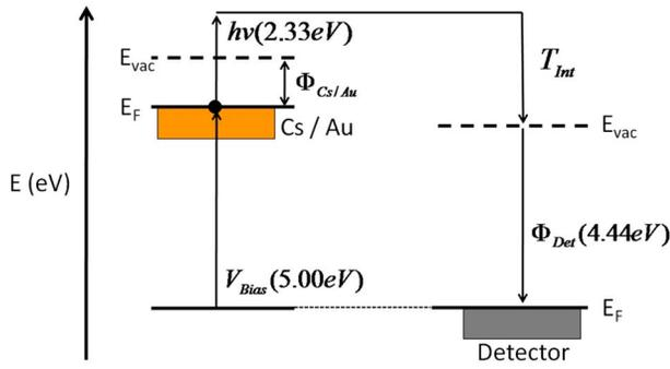
FIG. 1. (Color online) Energy diagram of a photoelectron. It is initially excited by a photon ( $h\nu$ ) into vacuum and then accelerated by a 5 V bias. The kinetic energy of the electron must be large enough to overcome the work function of the detector. The energy that is measured is the internal kinetic energy ( $T_{int}$ ).
