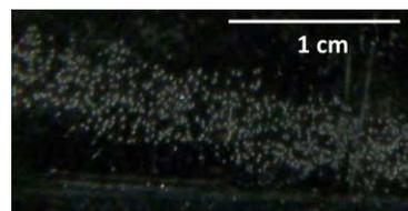
FIG. 1. Bubbles form along the laser beam line in response to a single laser pulse. The supersaturation was  $c/c_{\text{sat}} = 2.50$ . The laser produced 280 mJ/pulse at a wavelength of 532 nm, far above the threshold for laser-induced bubble nucleation.
