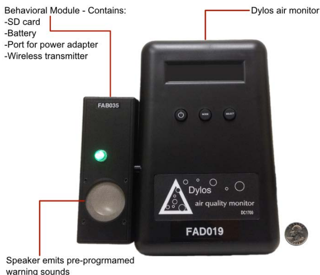
Figure 1. (Color online) Modified Dylos DC1700 Air Quality Monitor. Coin included to show scale
