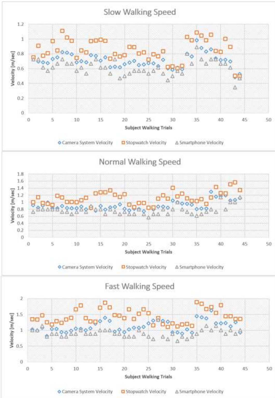
Figure 5: Walking speed trials measured concurrently through systems: 1. Camera system 2. Stopwatch and 3. Smartphone
