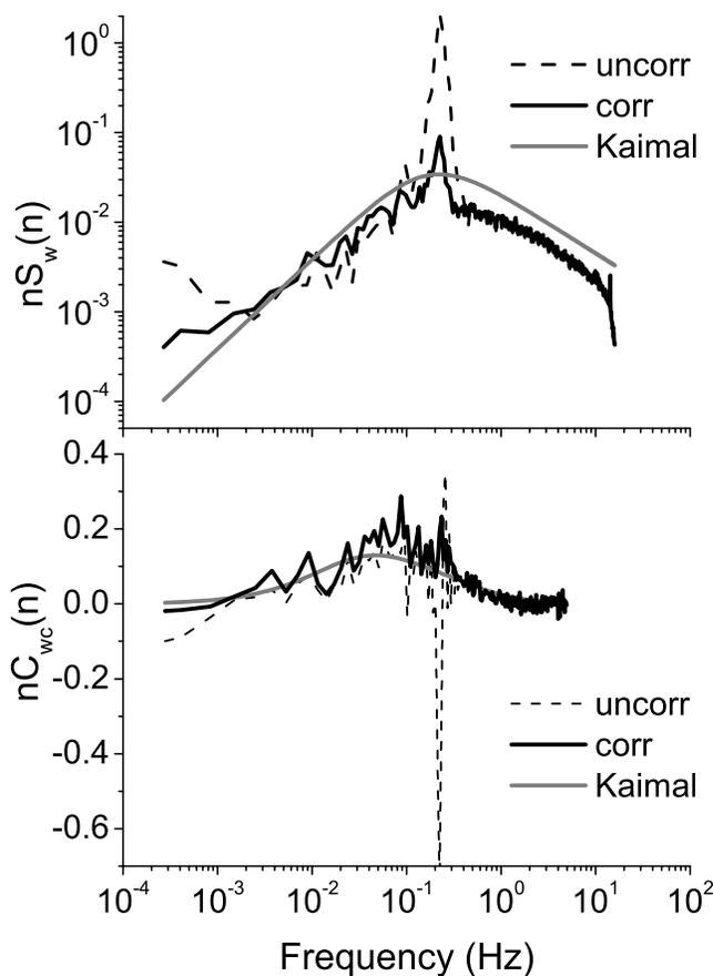
**Figure 6.** Effects of motion correction on (top) vertical wind power spectrum (50 Hz sampling frequency) and (bottom) DMS cospectrum (10 Hz sampling frequency). Dashed and solid lines are the uncorrected and corrected spectra. Shaded lines are computed spectra after *Kaimal et al.* [1972]. Data are from DOY 147,  $8^\circ\text{N}$ .
