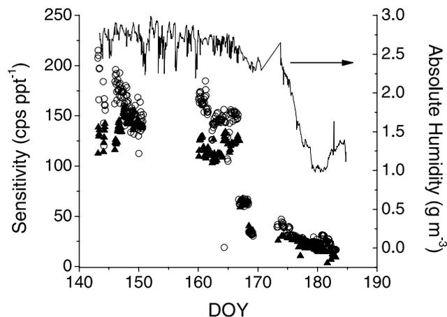
**Figure 5.** API-CIMS instrument sensitivity for DMS during the PHASE 1 cruise, determined from air (solid triangles) and water (open circles) analyses. Absolute humidity during PHASE 1 is plotted as a solid line (plotted on right axis).
