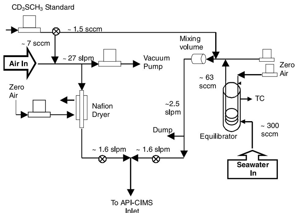
**Figure 2.** Schematic of API-CIMS experimental setup. On the left is the air sampling side and on the right is the water sampling side. Flow rates are given in standard cubic centimeter per minute and standard liter per minute.
