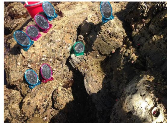
**Figure 2.** A single limpet-heating experiment. The experimental subject limpet is illuminated (bottom right) with 8 hand mirrors (upper left). The control limpet remains in the shadow of the adjacent substratum.
