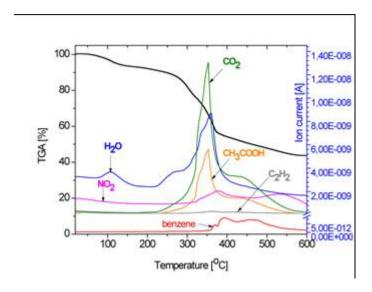
3 Figure 3. Spectra obtained from the thermogravimetric (TG) and mass spectrometric (MS)
