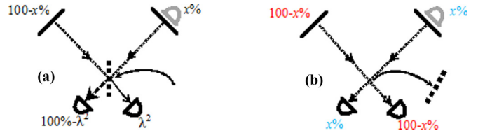
FIG. 4. (Color online) WM with a delayed-choice option. The transmission coefficient of the BS arbitrarily differs from 50%. (a) Interference upon the split photon’s return to the BS proves that the photon has remained superposed despite the weak which-path measurement. (b) BS removed before the photon returns. The two lower detectors confirm the weak measurement outcome.
