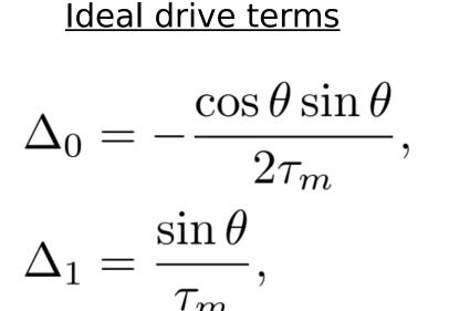
$\Delta_0$  - constant drive coefficient  $\Delta_1$  - linear feedback coefficient
