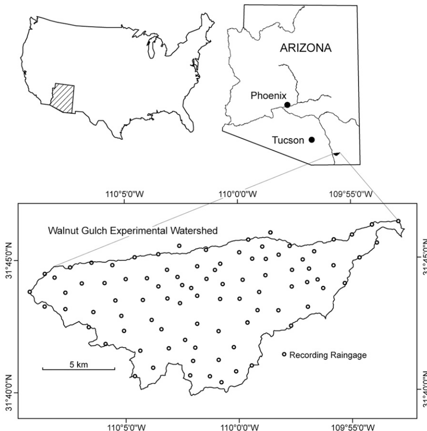
FIG. 1. The USDA-ARS Walnut Gulch Experimental Watershed (WGEW) location. The network consists of 88 weighing rain gauges within a 149 km 2 area.
